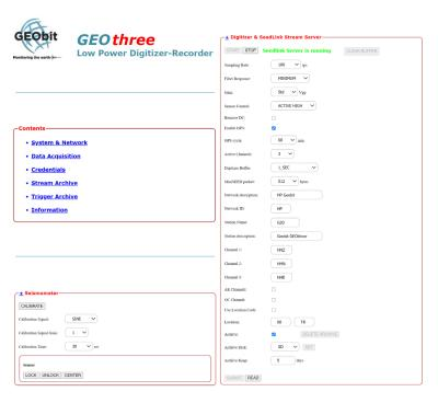
day solution to the user. The hardware is based over an embedded ARM9 400MHz ARM linux board running 14.6 linux kernel. The data are stored in mini-SEED format into the microSD card or to a removable USB stick. The instrument supports 10/100 ethernet port and debug port. FTP, SFTP, SSH are also available. The state of health is transmitted over UDP packets upon request.
