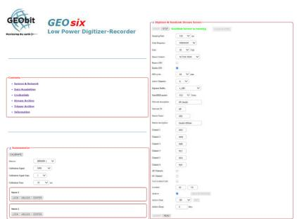
preamplifier. Our force-balance sensor front end is also supported, providing a wide-band response (10sec-98Hz) and high sensitivity 1500V/m/s by connecting a C100 sensor. Acquisition parameters and operation modes can be set from the user-friendly web interface, up to 64 characters password protected.
